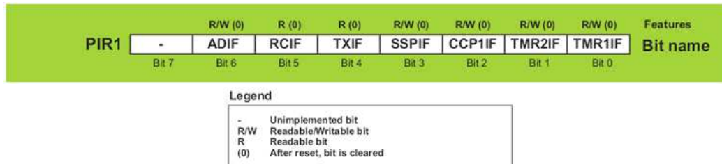
Fig. 2-13 PIR1 Register
